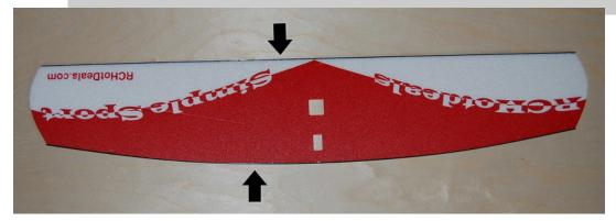
Glue the 3mm carbon strip to the front and back of the wing using med CA. Trim any overhang of the carbon with a sharp pair of wire cutters.
